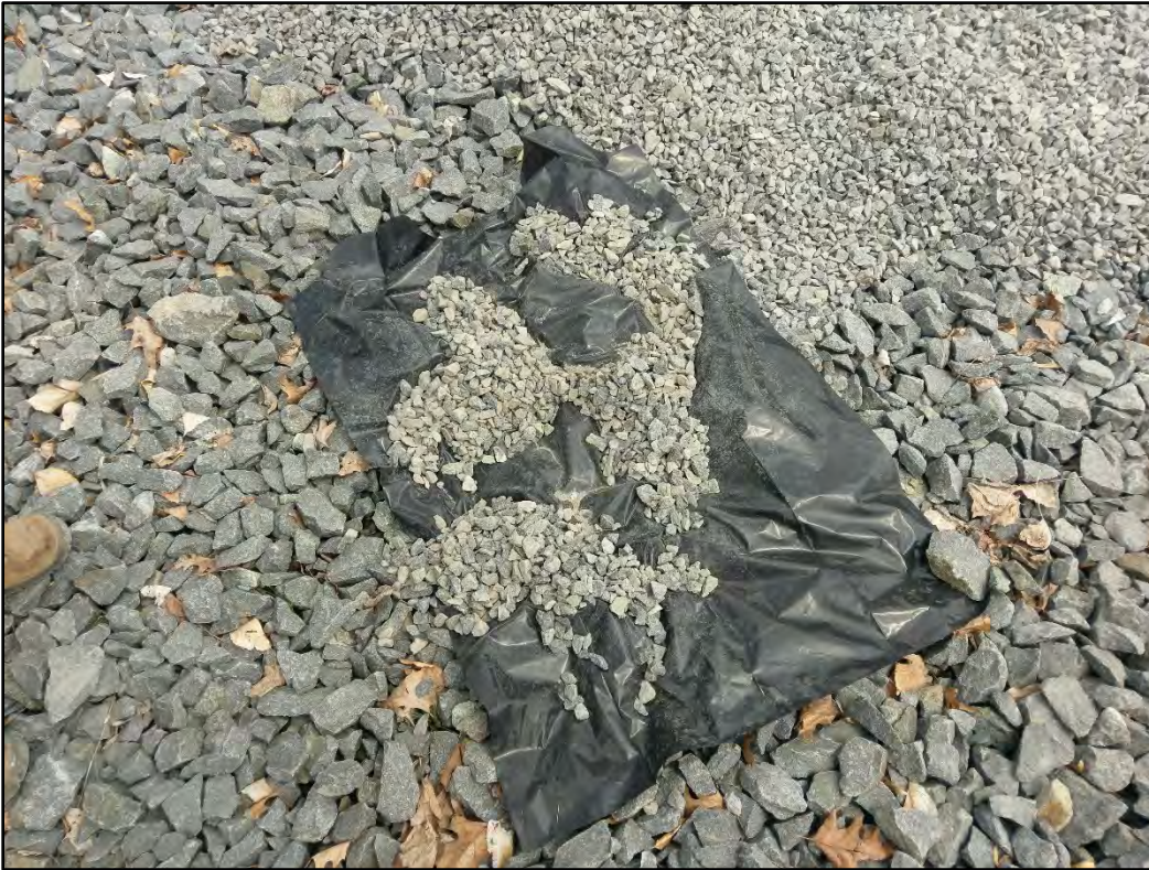
Photograph 6: One quarter retained, one quarter split with PA DEP, and two quarters discarded.
