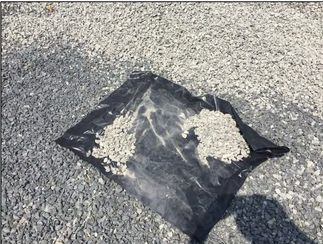
Photograph 6: One quarter retained, one quarter split with PA DEP, and two quarters discarded.
