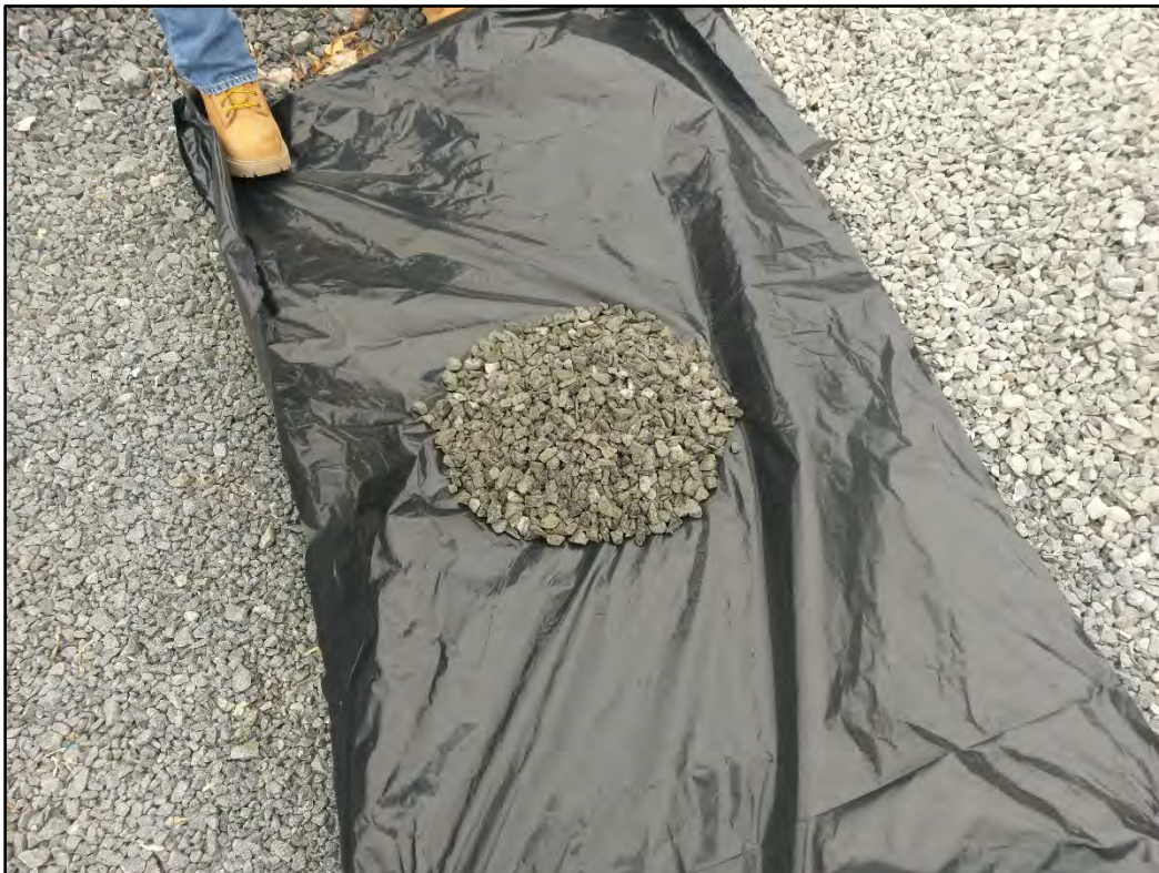
Photograph 4: AASHTO method, mix the four increments (one from each quadrant).
