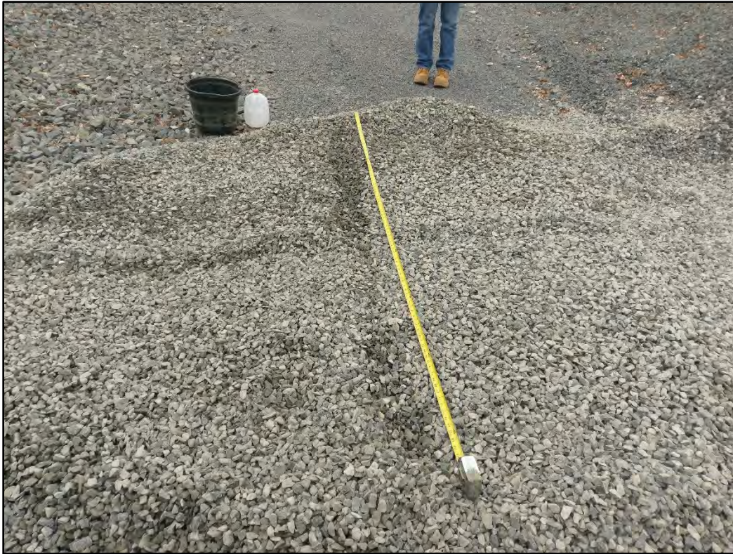
Photograph 4: AASHTO method, mix the four increments (one from each quadrant).
